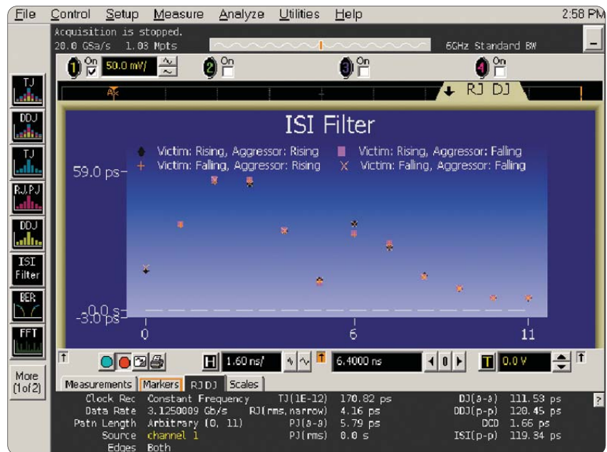
Figure 7. EZJIT Plus modeled the example signal's DDJ with this ISI filter when the lead value was set to 0 and the lag value was set to 11.
